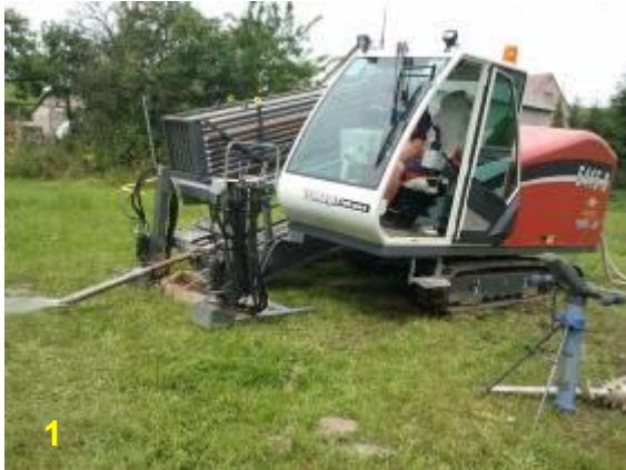
1 TJ 5415 S during the starting of the pilot bore.
