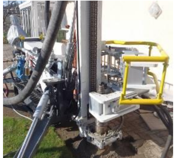
The triplex clamping and breaking system.
