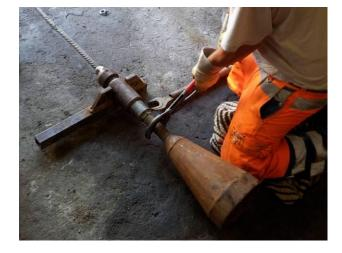
The TERRA-EXTRACTOR X 400 starts to pull in the expander cone.
