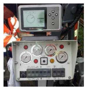
The control station and the monitor of the locator. The operator sees all relevant data.
