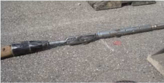
← The bursting tool consisting of the roller cutter 2", the extra large cutting roll and the expander cone Ø 100 mm (4").
