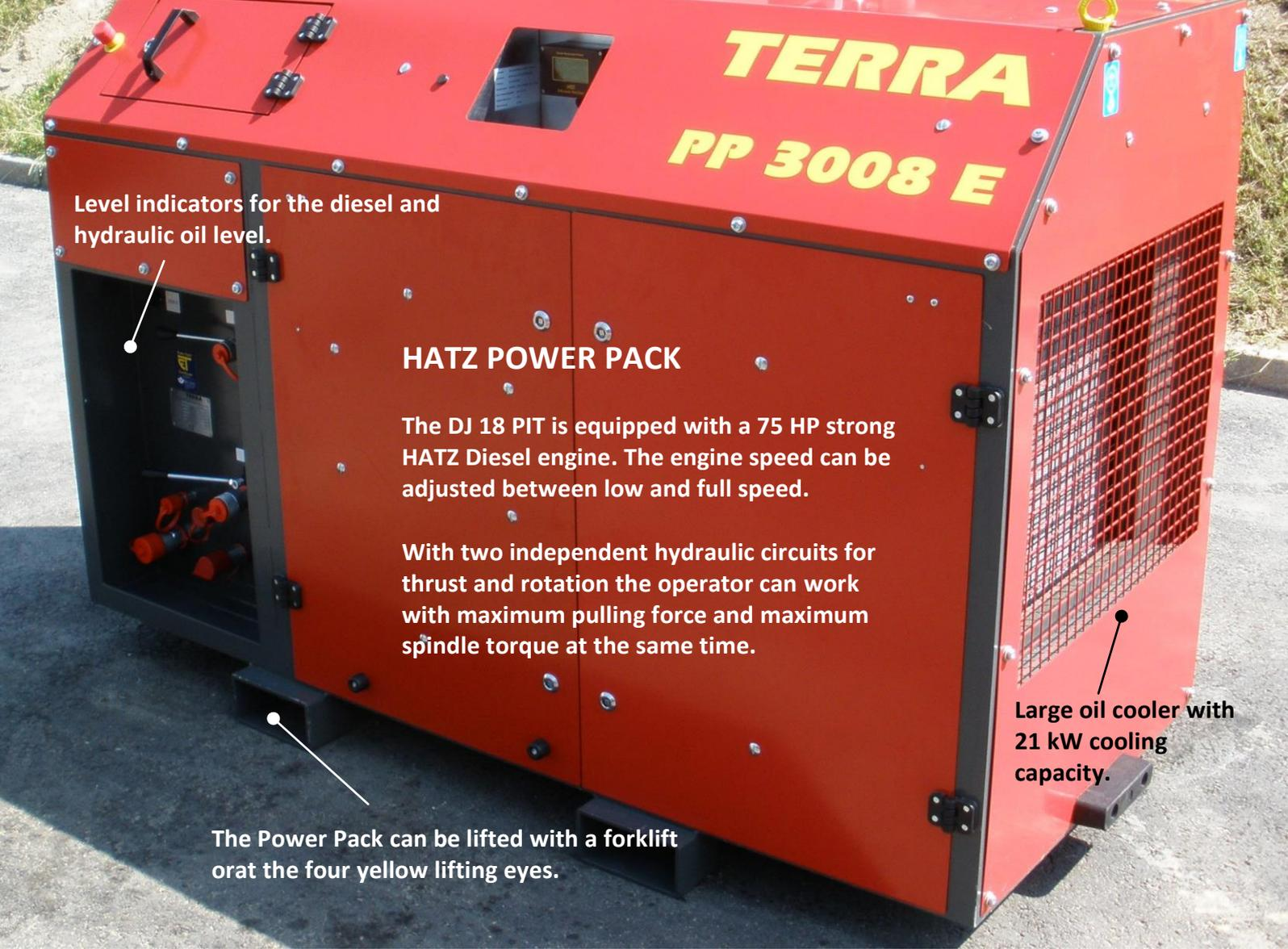
Level indicators for the diesel and hydraulic oil level.
