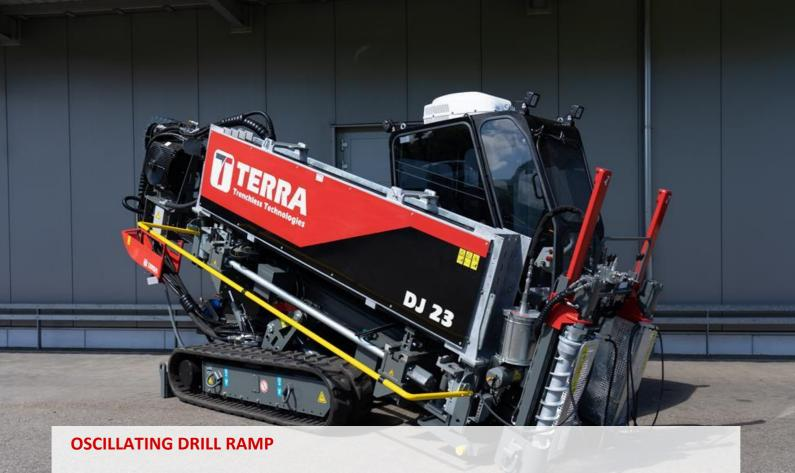
TERRA has developed a patented oscillating drill ramp for the DJ 23. It has two rotation points with two separate cylinders. With this unique system, the drill ramp can achieve a drilling angle from **19** % **up to 40** % (11° - 22°). The rubber crawler stays firm on the ground up to a gradient of 36%.
