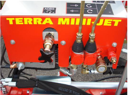
The star knob adjusts the ADBS II pressure. The right knob adjusts the drill rod rotation speed.
