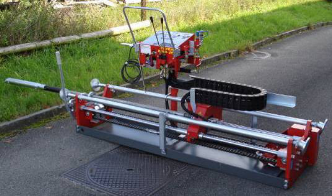
The drill rig TERRA MINI-JET MJLV 1600 with drill head
