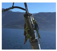
**STEEL PIPE RAMMING APPLICATIONS** The TR 200mini rams steel pipes up to  $\emptyset$  150 – 400 mm over lengths of 30 m. Vertical or horizontal application possible.
