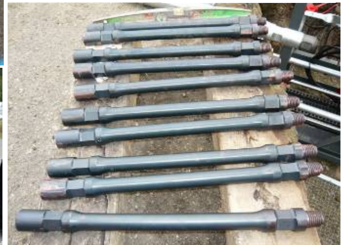
↓ The special drill rods of the TERRA MINI-JET allow minimum turning radiuses of 15 m (50"). This is unique world wide.
