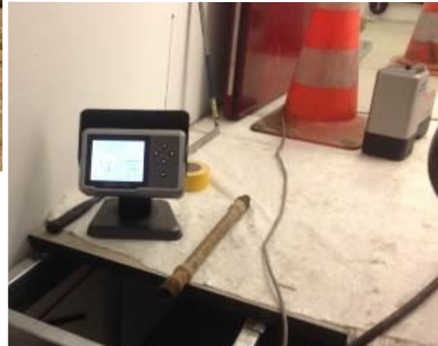
→ The monitor (display) shows all relevant data. The locator (receiver) stands at the right side.
