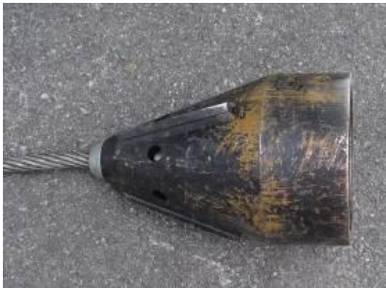
The cable burster with bent front plate is ready for installation in the manhole \varnothing 800 mm (32").
